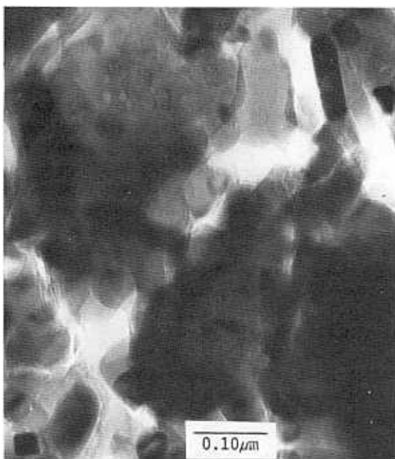
Figure 8: TEM of sections of 3Al 2 O 3 :1B 2 O 3 :3SiO 2 fibers fired at 1200°C for 1 hour.
