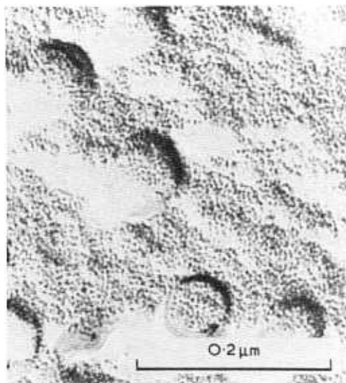
Figure 7: Replication electron micrograph of 18.6 mol % soda gel glass after heat treatment at 710°C for 1 hr. Reproduced from Reference 13.
