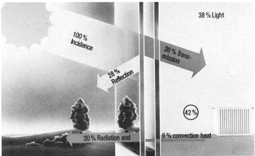
Figure 20: IROX A1, medium. Balanced properties of reflection and transmission. IROX facade panels particularly suited for all-glass facades.
