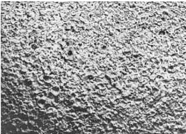
Figure 27: Surface of a light-scattering coating.
