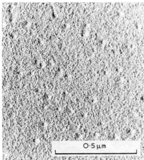
Figure 8: Replication electron micrograph of 18.6 mol % soda gel glass after heat treatment at 755°C for 10 min. Reproduced from Reference 13.
